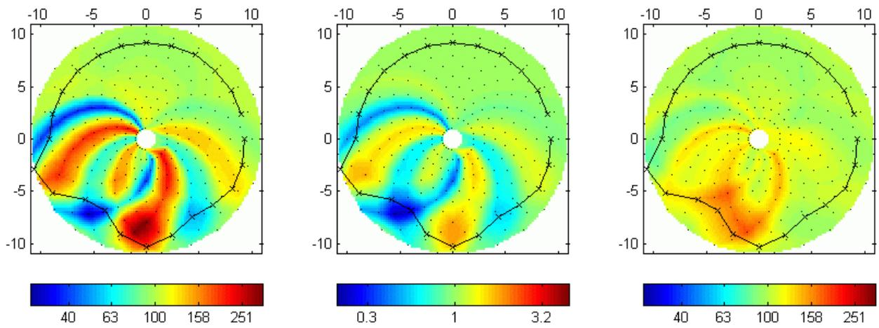
Abbildung 2: Raw data (left), topography effect (center) and corrected data (right) for the synthetic model
